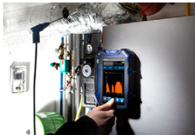
Spillage Test Optional probe available to test for back-draught conditions in the chimney.
