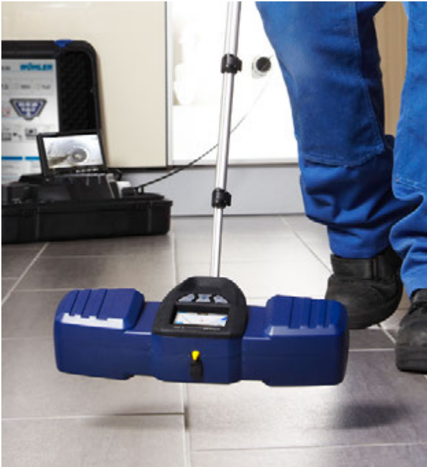
Acoustic and visual signals: the Wöhler L 200 makes it possible to locate the camera head.
