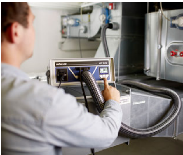
Leakage tests on several 100 m 2 of installed ductwork systems.
