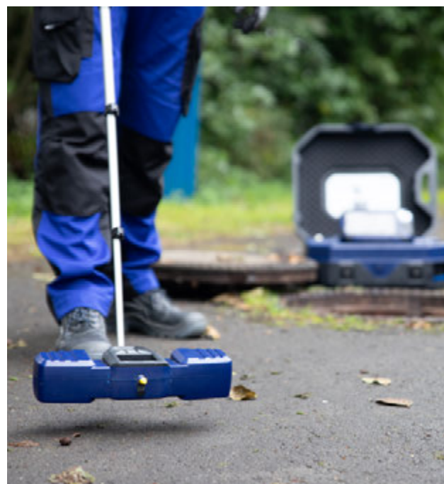
With the Wöhler L 200 Locator, the camera head can be located with pinpoint accuracy.
