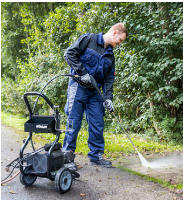
Cleaning with the lance - choice between 5 nozzles is possible.
