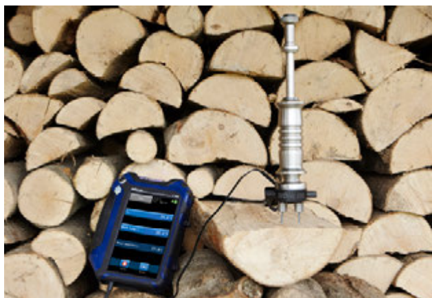
Wood Moisture Measurement Optional probe available for wood moisture measurement.
