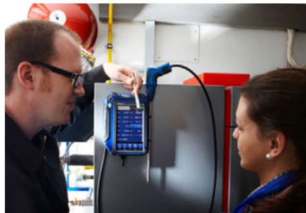
Large 7" color Touchscreen All results of measurement at a glance – Use the large, clearly arranged color touchscreen to explain the results.
