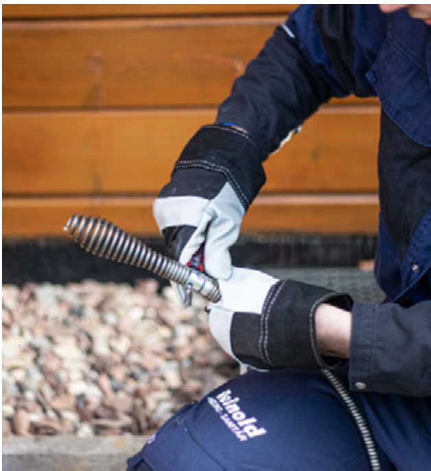
Easy and quick change of the drill heads.
