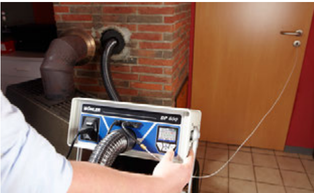
4 Pa-Test with low pressure measurement and data logging.
