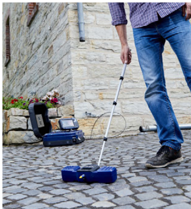
Precise location of the camera head with the Wöhler L 200 Locator.
