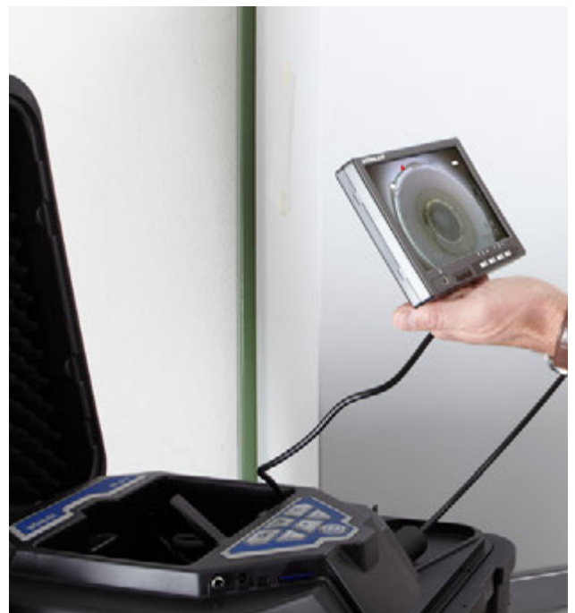
Tiltable and removable TFT wide-screen color monitor.
