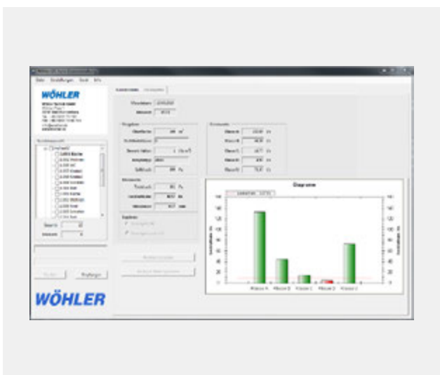
Wöhler DC Series PC software for data transmission and subsequent processing (optional documentation set).
