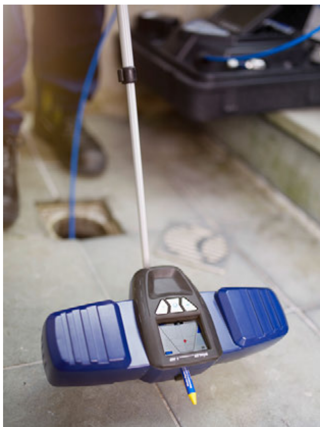
The Wöhler VIS 350 precisely locates radio waves transmitted by the camera head through concrete and asphalt to save a lot of time and further building damage.
