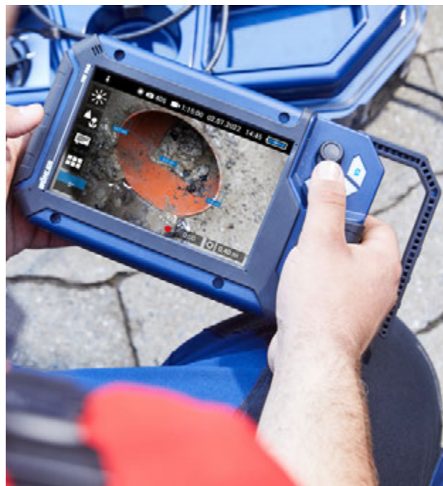
Focus adjustment and distance measurement: The measurement function allows to determine the distance between the lens and a selected point or between two selected points.
